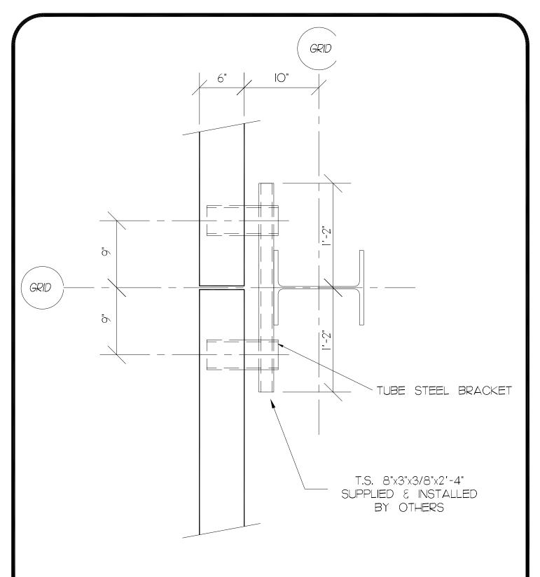
PANEL BEARING TO STEEL COLUMN
